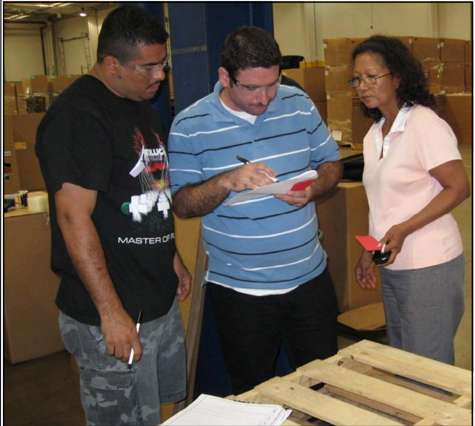
A 5S check list prompts Hi-Tech employees to look at a work area with fresh eyes. Any item not essential to production—box, broom, tool—gets a red tag and moved out.
